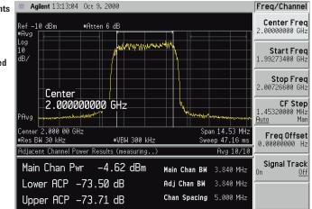
The usable dynamic range of the PSA is enhanced by a standard 2 dB step attenuator that covers the complete frequency range of the analyzer, and by the ability to switch off ADC dither to lower displayed-average noise level (DANL).
